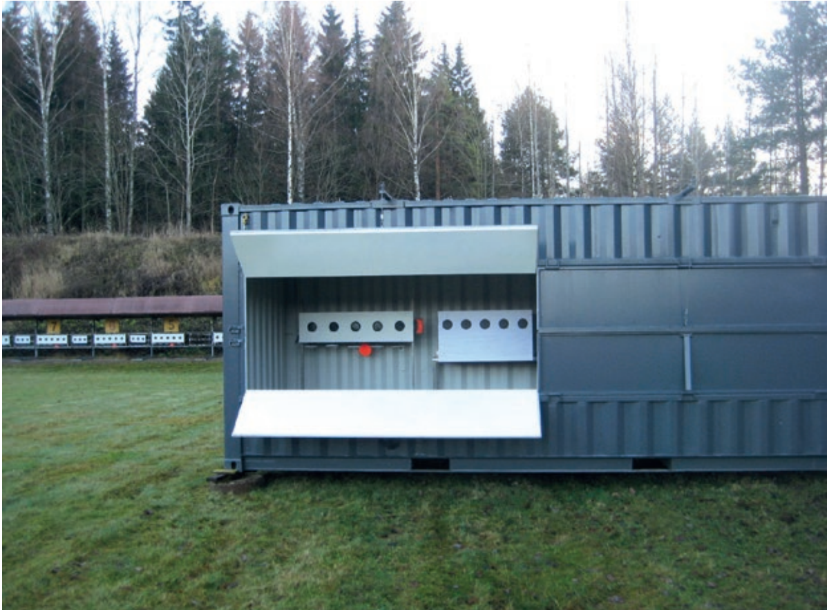
Figure 5.11. Biathlon target equipment and bullet traps installed in a shipping container, prototype (photo: Pauli Harjula).
