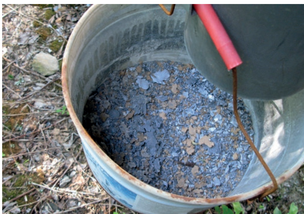
Figure 5.8. Fragmented bullets from steel bullet traps.
