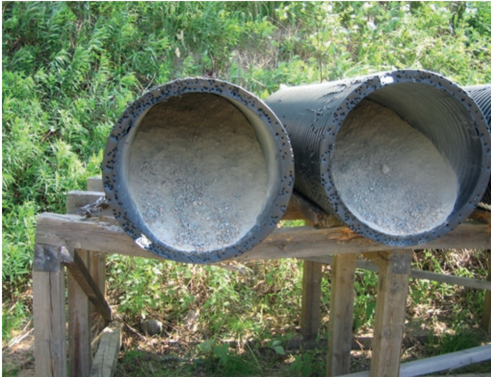
Figure 5.10. Bullet traps at the Koivujärvi pistol shooting range (photo: Finnish Defence Forces).
