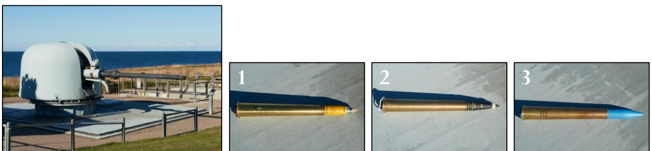
Figure 11: 76 mm OTO Melara with different ammunitions. (1) 76 mm High Explosive (HE), (2) 76 mm Sapomer, (3) 76 mm Training Projectile.
