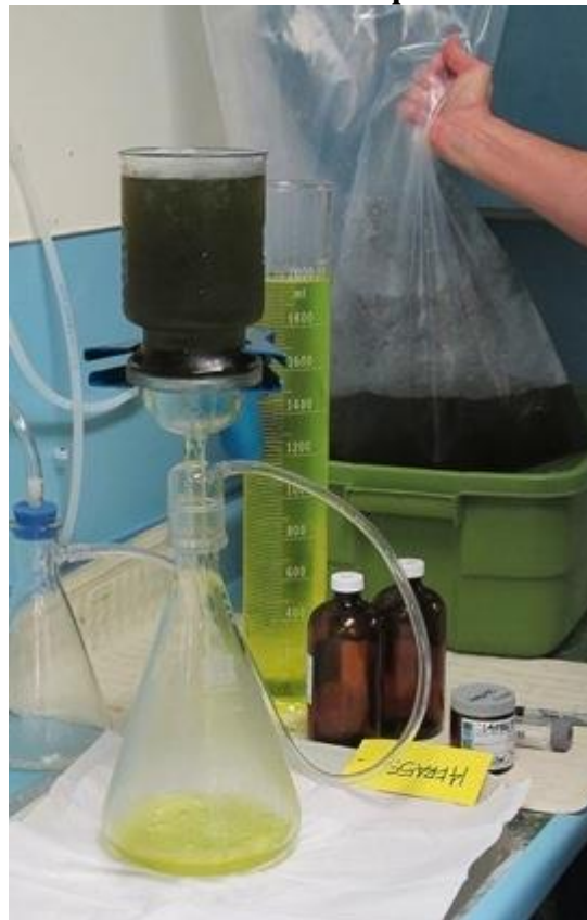
Figure 4. Separation of the solid and aqueous phases of the melted post detonation samples.
