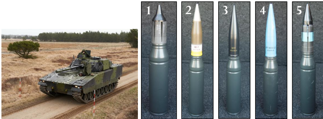
Figure 2: 35 mm Bushmaster Cannon on Combat Vehicle CV9035 with different ammunitions.
