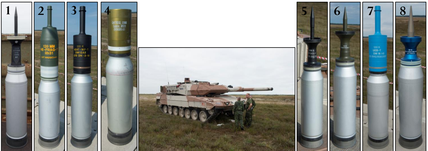
Figure 6: 120 mm Rheinmetall L55 Smoothbore Gun on Leopard 2 A5 with different ammunitions.
