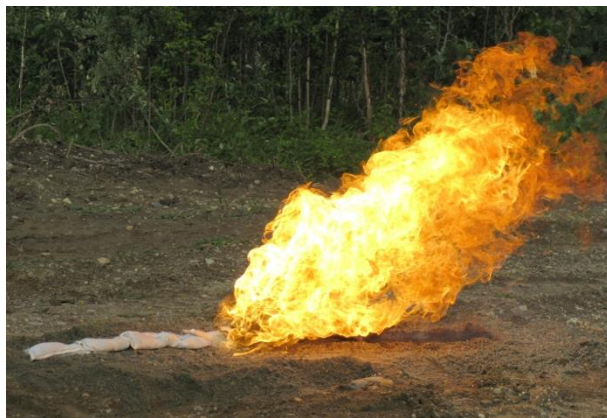
d. Burning a line of propellant on soil (4)
